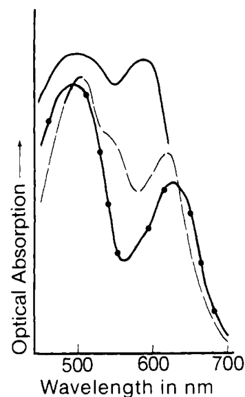
Figure 1. Solid state absorption spectra of cyanine-oxonol dye salts. The spectra were obtained as Nujol mulls: Ia (---), Ib (---), and Ik (—).
